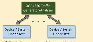
Multiport traffic generation and analysis as end point device. (1ns precision latency measurement)
