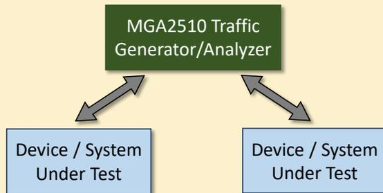
Traffic generation and analysis as end point device. (1ns precision latency measurement)
