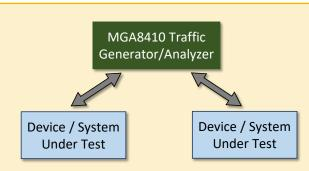
Traffic generation and analysis as end point device. (1ns precision latency measurement)
