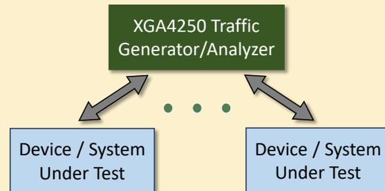
Multiport traffic generation and analysis as end point device. (1ns precision latency measurement)
